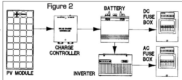
a battery bank, a DC fuse box, an inverter, and an AC fuse box. (See Figure 2.) Functionally, the PV array and charge controller together are no more than a simple battery charger that uses sunlight as its energy source.
